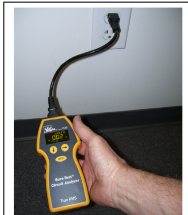
USE CIRCUIT ANALYZER TO CHECK CIRCUIT LOAD
